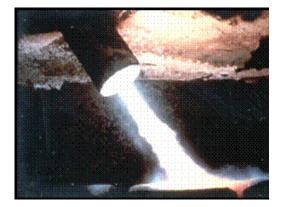
Photo 1 Transferred Plasma-Arc Torch Courtesy Plasma Energy Corporation
