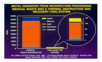
Comparison of Emissions-Incineration vs. Plasma Pyrolysis
