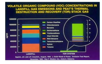
Comparison of Landfill Emissions vs. Plasma Pyrolysis
